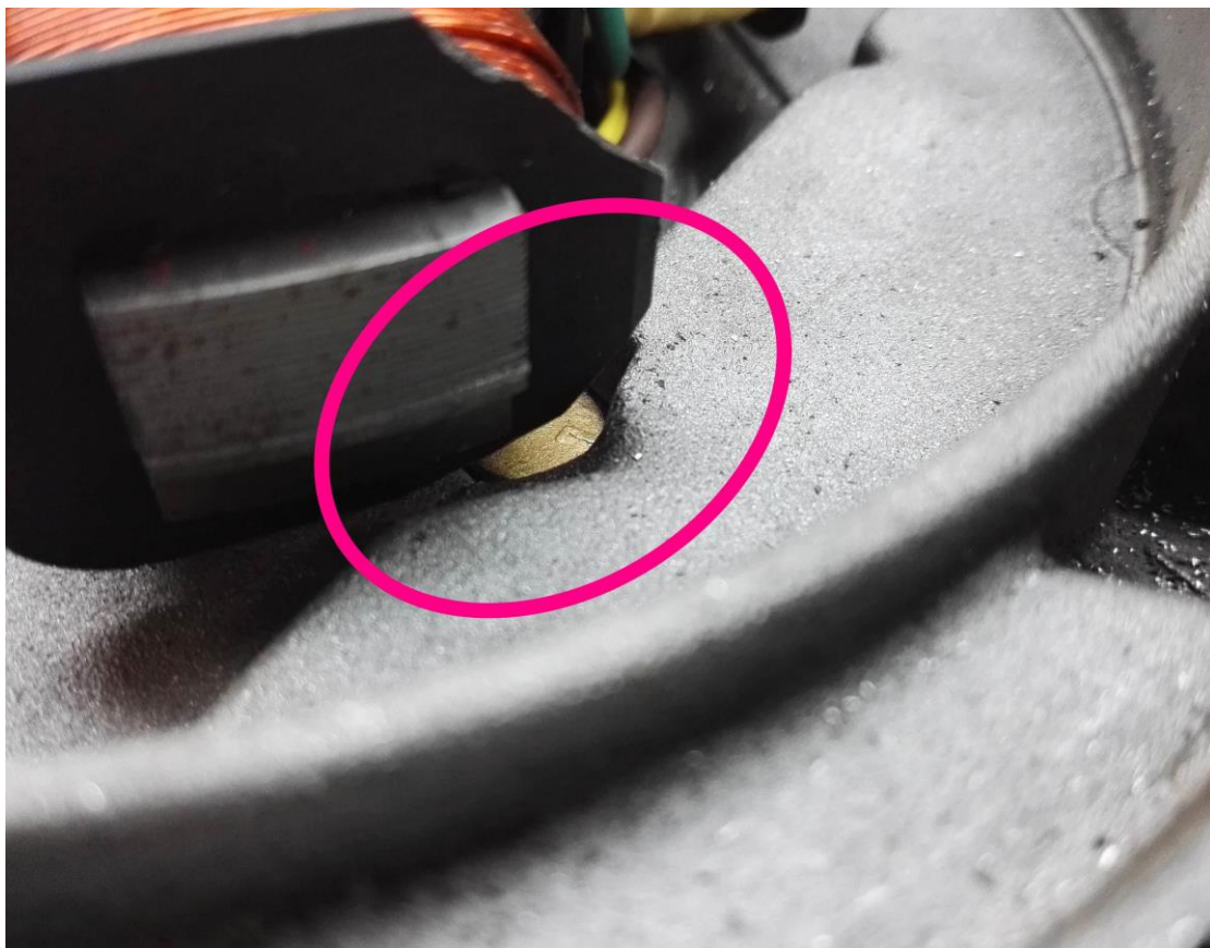
Modification of the coil's plastic, because it touch on the carter. Beware to not damage the coil wire winding.
